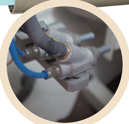
Double Venturi guns with Tungsten Carbide nozzles
