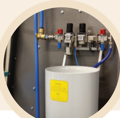
Optional 45 litre pressure pot attachment for detailed hand work
